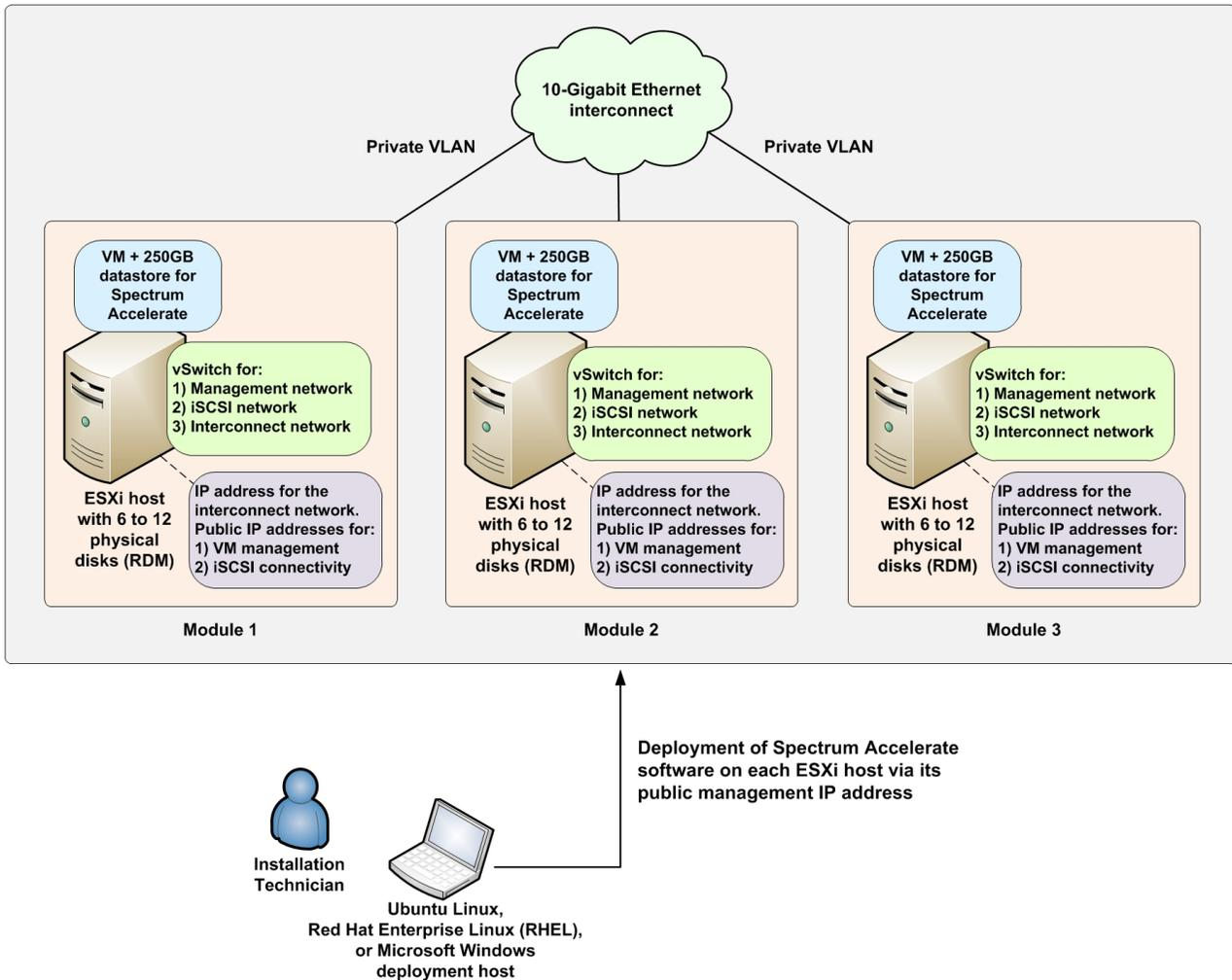
Figure 2. Visualization of the ESXi configuration and Spectrum Accelerate software deployment
