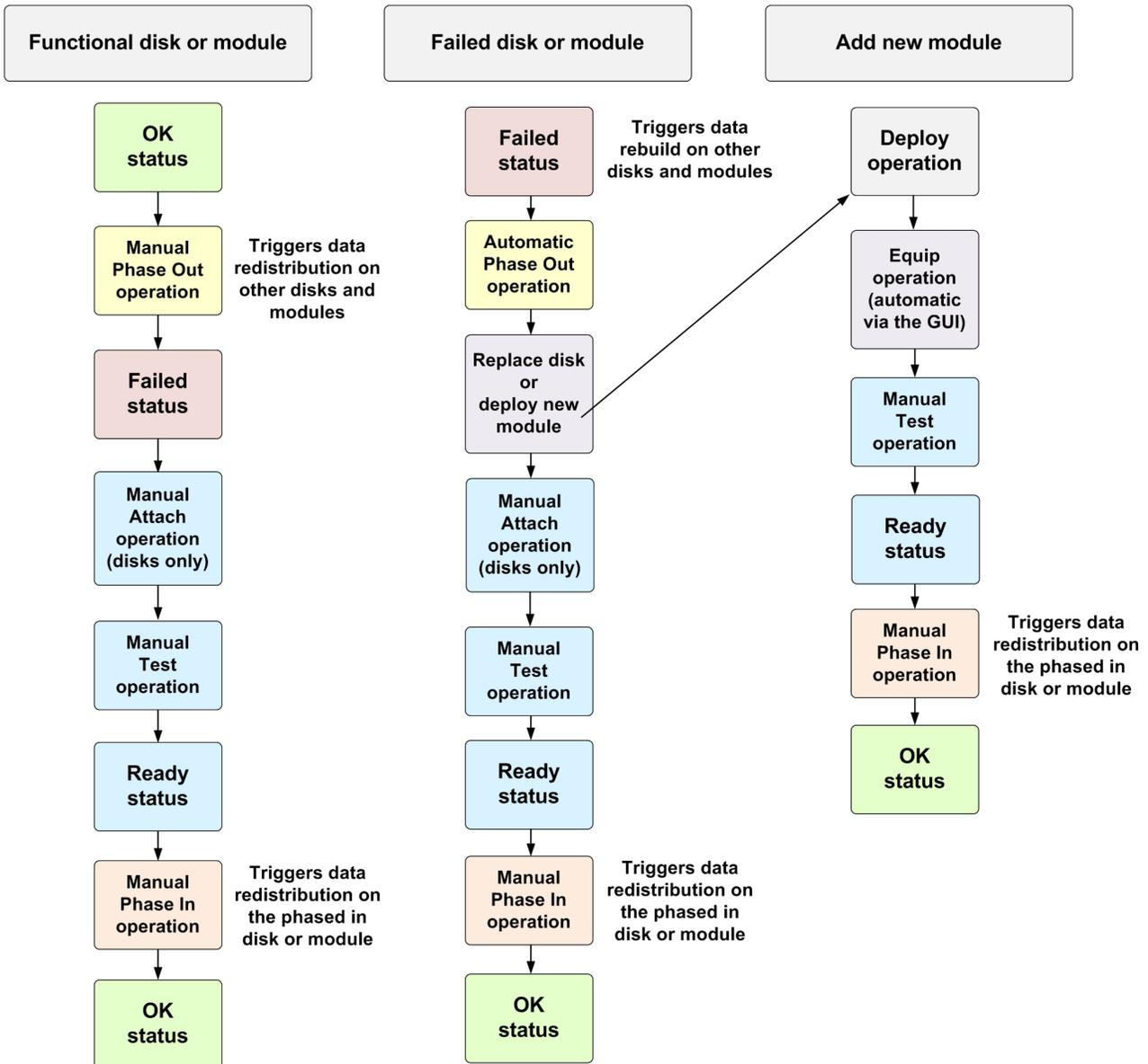
Figure 65. Flowchart of hardware service operations and statuses
