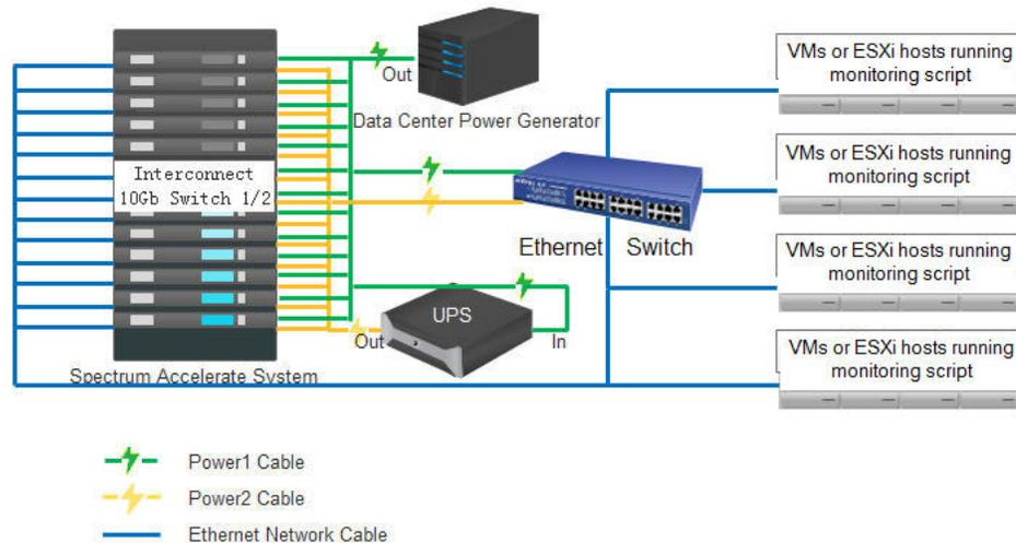
Figure 77. Power supply monitoring architecture with a non-Smart UPS unit
